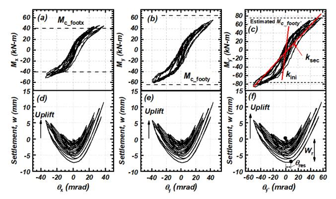
Figure 4. Results of test SE03 (a)  $M_x$  vs.  $\theta_y$  and w vs.  $\theta_y$  and (b) My vs.  $\theta_x$  and w vs.  $\theta_x$  and (c) resultant moment ( $M_R$ ) vs. rotation ( $\theta_R$ ) and settlement (w) vs. rotation ( $\theta_R$ ) for test OE03.
