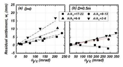
Figure 7 Normalized residual settlement vs. cumulative footing rotation of the footings grouped into different A/Ac ratios.
